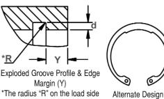
Ch Max Allowable Corner Radius & Chamfer
