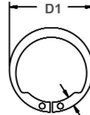
Measuring Free Diameter (Df) SHI Series Df = D1 - 2(S \text{ max})
