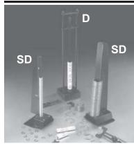
**Retaining Ring Dispensers** Rotor Clip retaining ring dispensers feature "rail" over which a stack of retaining rings can be slipped. Once in position, they can be "dispensed" one at a time using a retaining ring applicator for ease of installation. Two such models are available to meet you particular dispensing needs: **Spring Rail (SD)** dispensers are competitively priced and offer significant improvements (like more rail capacity and durable construction) on existing designs.
